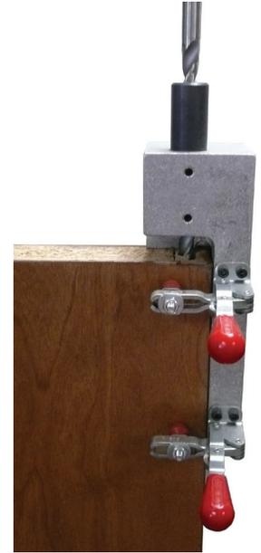
The Extension Flush Bolt Drill Fixture is designed to drill a 1/2" diameter hole up to 16" long in a door for the extension rod on a flush bolt. The unit is primarily designed to be used on 1-3/4" thick doors and to position the center of the hole 3/4" from the door edge. Shims can be used for applications on thinner doors or if the hole location is to be less than 3/4" from the edge.
