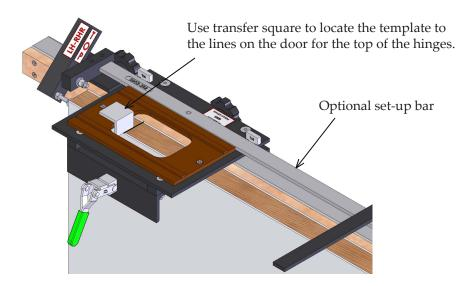
When measuring on the HS 3000 itself, it is most convenient to measure to the center line of each hinge which is scribed on each template holder. Measure from the near side of the end stop cross piece. End stops are accurately adjusted at the factory, but may be checked by locating a template holder in this way and then checking its location with the transfer square.
