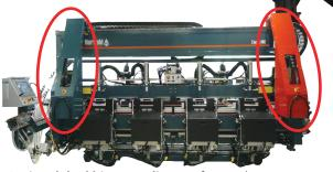
**Optional dual hinge applicators** for quick change between 3-1/2" and 4" hinges.
