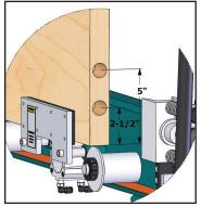
Quick change adjustment for drilling 2-1/2" to 5" from door edge.
