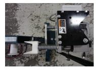
Self-centering mechanism enables drilling I-3/8" to I-3/4" thick doors with out any adjustments.
