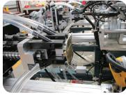
Fully Automated Hinge Application: standard hinge applicators install 2 or 3 hinges simultaneously.
