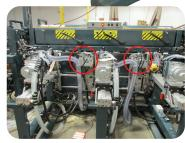
**Standard Automatic Predrills:** ensure hinge screws are straight and do not split stile or jamb.
