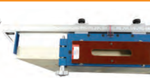
The end stop can be adjusted for different header clearances
