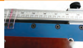
Centerline pointer aligns with scale for positioning fixtures
