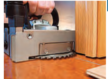
Cut door frames without disassembling the butt straps.
