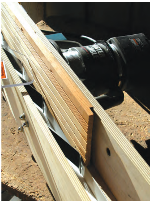
Special stepped cutter cuts backstop and makes kerf in one pass.
