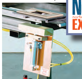
Jambs are held securely with foot-operated air clamps under each template.
