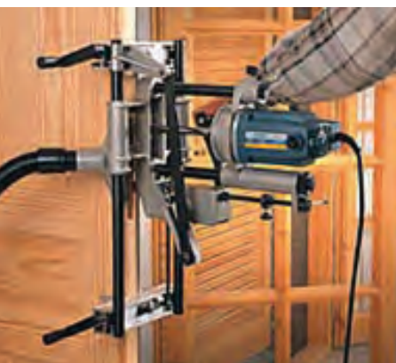
A locking bar can be placed at a fixed height for multiple doors of the same height.
