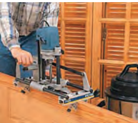
A locking bar can be placed at a fixed height for multiple doors of the same height.
