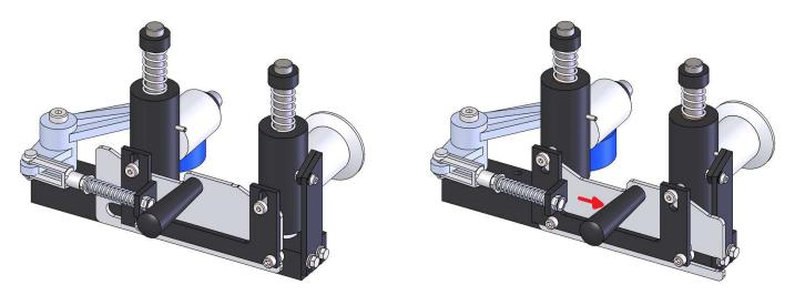
• Second, adjust the infeed bed up so that the door will pass over the beveller cutter head. The support roller will prevent the door from dropping onto the cutter head when the door leaves the infeed bed.
