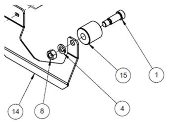
C. Using the 5/16" bolts and washers, mount the bracket, 6803-045, to the infeed bed.
