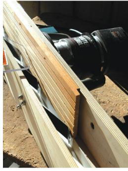
The Weatherizer is a dedicated door shop tool for preparing exterior door jambs for installation of weatherstripping.
